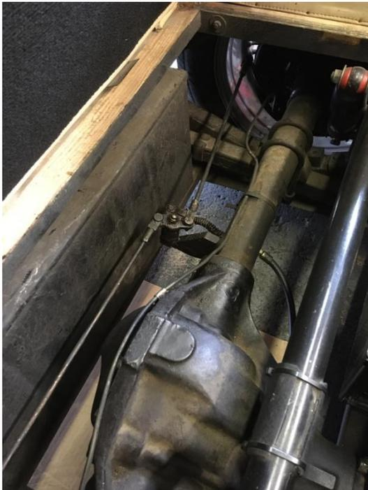
The issue would appear to be with pre 1996 Morgans fitted with the Salisbury rear axle - my car is a 1993 +4. After 1996 Morgan's began to fit BTR axels which have a different arrangement for the handbrake. On the Salisbury axel fitted by Morgan, the handbrake compensator linkage is mounted on a very substantial bracket welded to the rear axle. This arrangement provides very little clearance between the compensator linkage and the back of the fuel tank - Picture 1.
